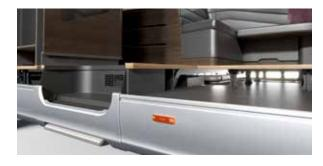
**DOUBLE FLOOR** \_ Single level floor throughout, with under-floor space, for integrated utilities, insulation and storage.
